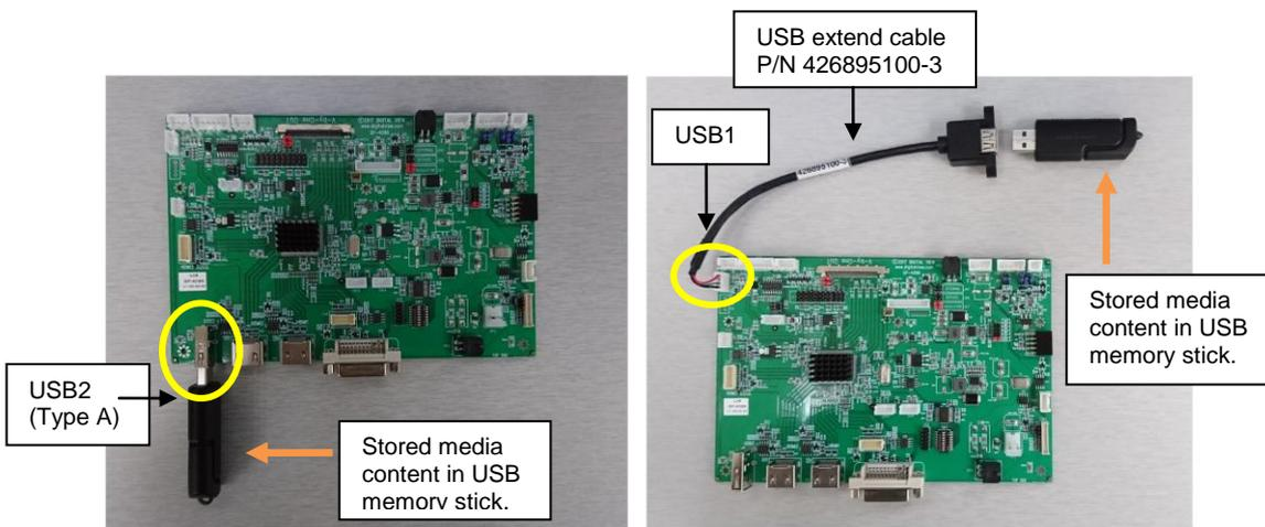
**STEP 3 :** The built-in media player will run and display the video content stored in the USB memory stick automatically if the video input source is no signal / loss of sync on a designated input.
